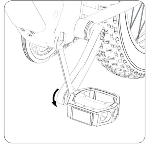
12. Use a wrench to tighten the pedal.
