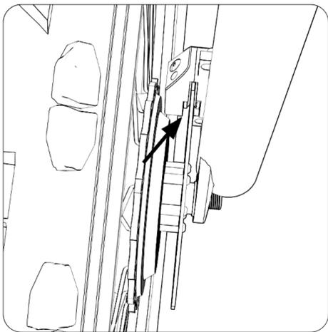
7. Note: Align the disc with the brake.
