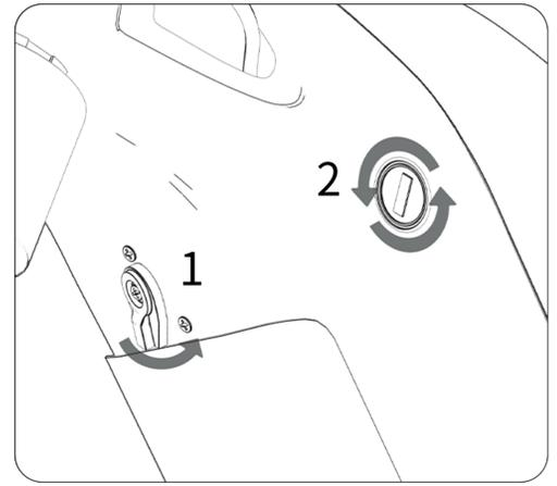
3. Twist the buckle to prevent it from falling. Turning the key to the "lock" position.
