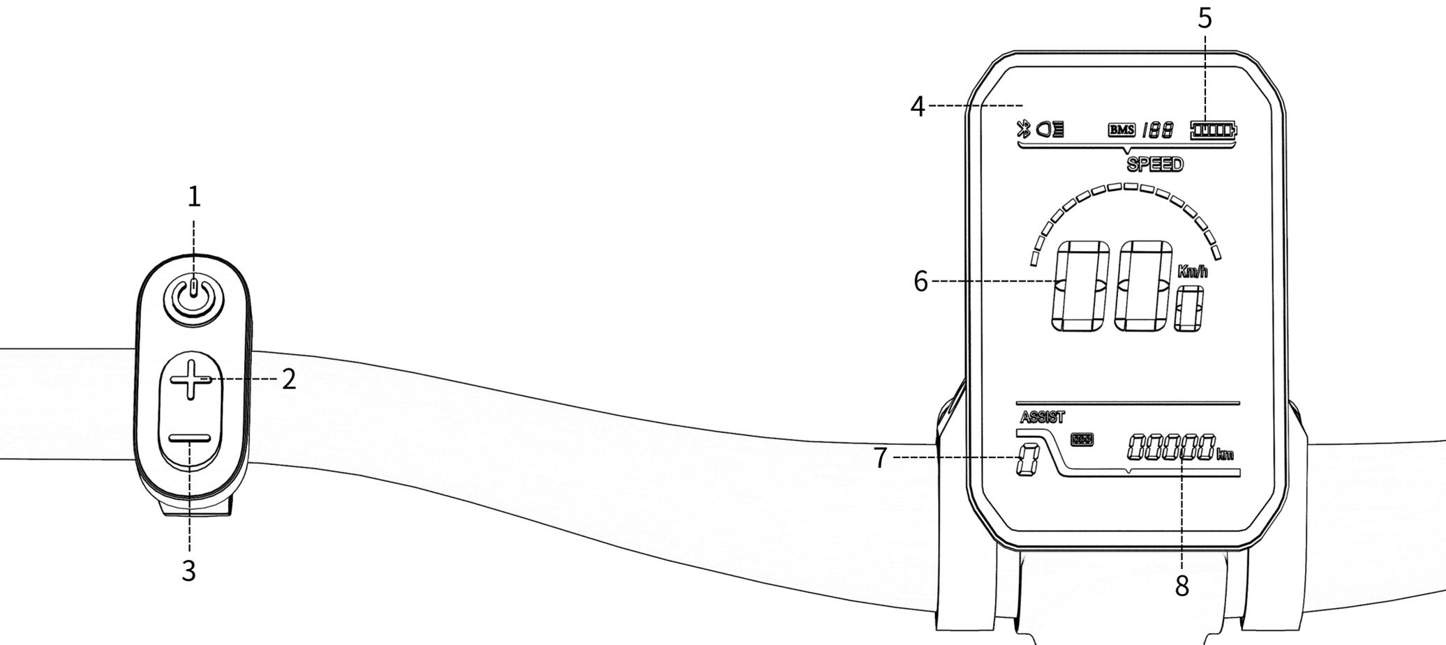
1. Switch on/off the Long button for 3 seconds to start
