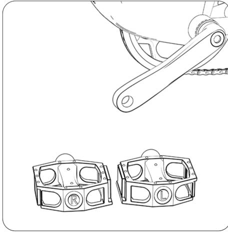
11. When installing the foot pedal, pay attention to distinguishing between "R" and "L".
