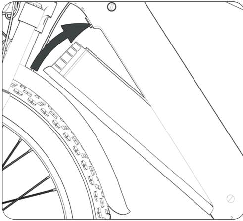
2. Connect the battery socket to the pin and push it up.
