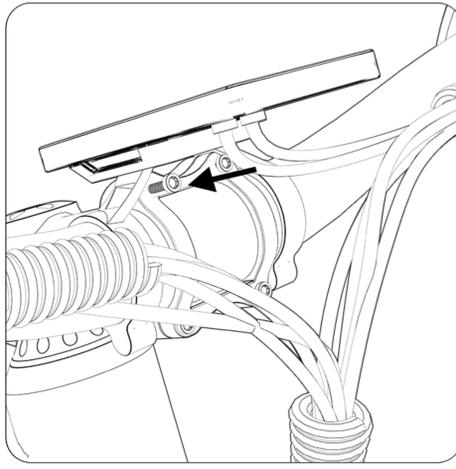
2. Attach the handlebar to the stem connection, and thread in the bolts.
