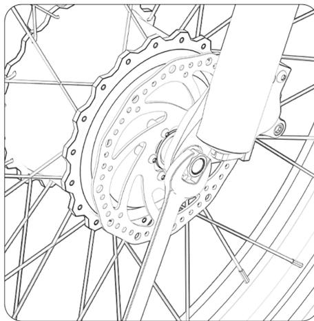
8. Use a wrench to tighten the screws.
