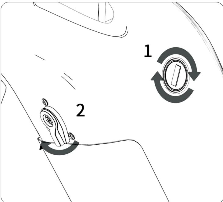
1. Unlock the battery with the key
