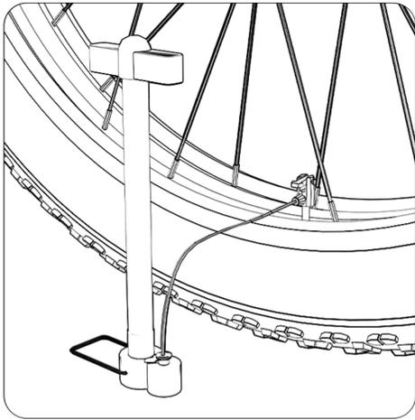
4. Inflate the front wheel slowly to prevent the tire from bulging out on both sides.
