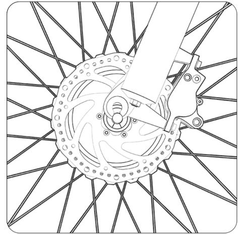
6. Front fork alignment motor shaft installation.
