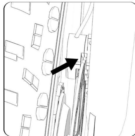
6. Note: Align the disc with the brake.
