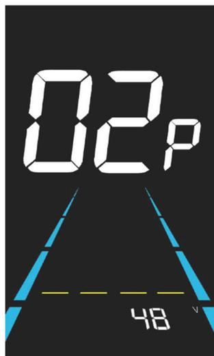
Figure 6-2 Rated voltage setting interface
