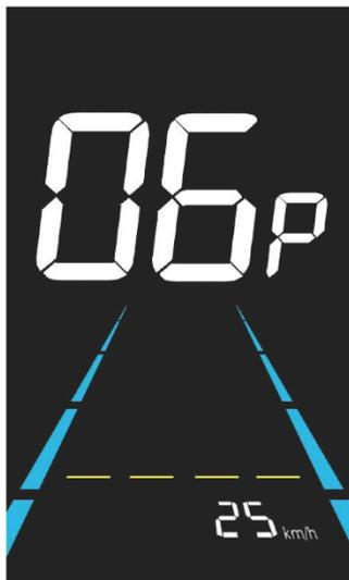
Figure 6-7 Speed limit setting interface
