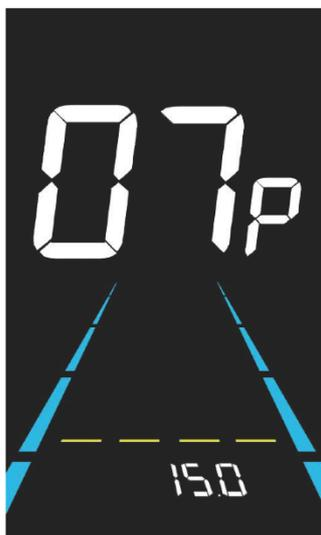
Figure 6-8 Controller current limit setting interface
