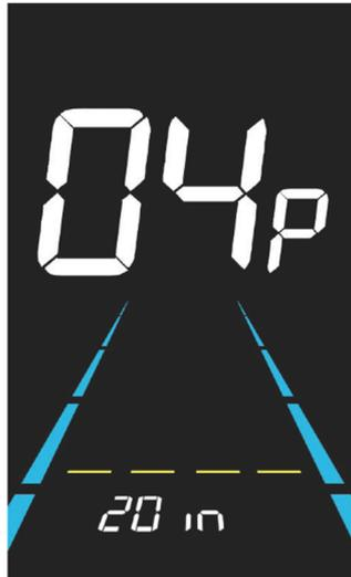
Figure 6-5 Wheel diameter setting interface
