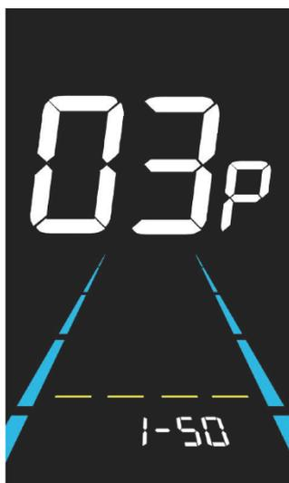
Figure 6-4 PAS level ratio value setting interface
