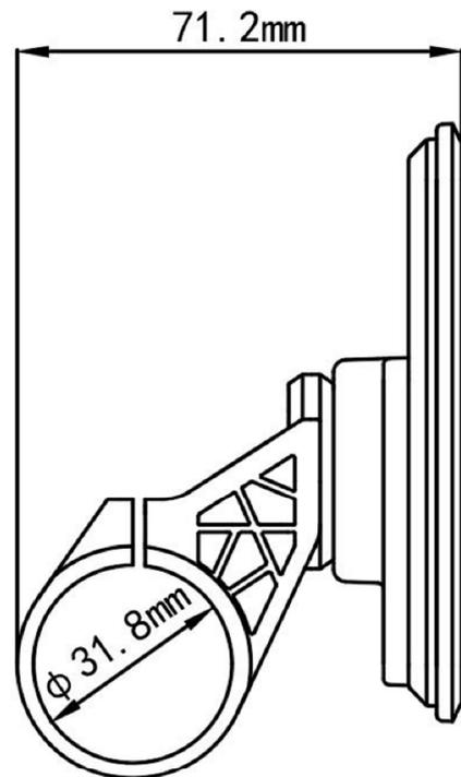
Figure 3-5 90T-V Side View Dimension
