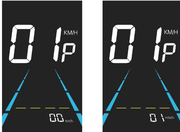
Figure 6-1 Metric and Imperial Units Setting Interface
