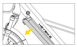
Turn the locking lever on the battery to the right and pull the battery down and away to remove the battery from its holding.
