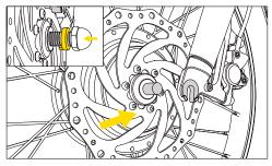
3 Remove the nut in the front wheel first. Install the front wheel axle into the front fork slot and secure it.
