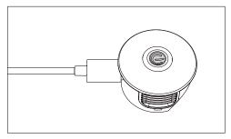
3 When the taillight LED flashes, it is charging. It is fully charged after about 1 hour.
