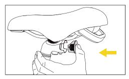
4 Remove the charging cable and with the taillight LED facing towards you, use both hands to push the light inward to install the taillight.
