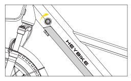
1 Ensure the bike is turned off. Insert the battery key, hold the top of the battery with one hand, and turn counter-clockwise towards the "unlock" icon.
