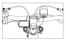
Place the handlebar onto the head part, adjusting the handlebar angle to ensure it is properly aligned with the bike.
