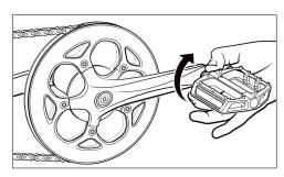
Thread the right pedal onto the right crank gently by hand, turning clockwise. Then tighten the pedal with an Allen wrench.
