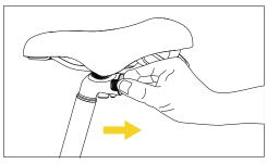
1 Hold both sides of the taillight and pull the taillight out from the bike to remove it.
