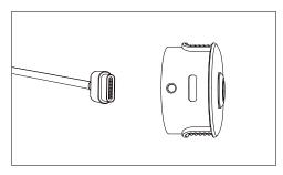
Connect the charging cable with the taillight charging port to charge it.
