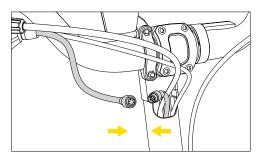
4 Like the headlight connection, insert the display cables into the hole and attach the green connectors according to the arrow direction markings. Press them together to connect.
