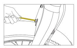
3 Align the fender with the screw hole then tighten the fender to the front fork.
