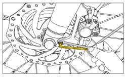
4 Use the screws from step 1 to install and secure the front fender bracket to the front fork.
