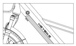
4 The outer battery cover should be flush with the bike frame.
