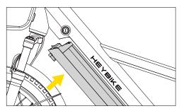
3 To install, insert the battery into the battery frame, bottom part first. The "bottom" is indicated by slots for connector ports. Pushing the top of the battery into place, a clicking sound will indicate the battery is properly in place.
