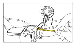
2 Put the headlight onto the handlebar and tighten the screws.
