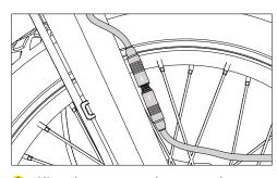
6 Align the arrows and connect the motor cables correctly.
