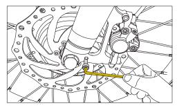
1 Remove the screws on the left and right sides of the front fork.
