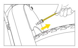
Remove the screw at the front of the front fork.
