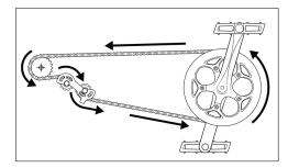
Check the chain alignment. Rotate the right pedal counter-clockwise. Watch the chain and ensure it runs through the drivetrain (the rear cog, chain tensioner, and around the front chain ring) smoothly.
