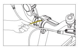
3 Tighten the stem screws.
