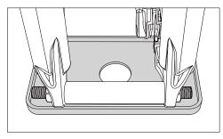
Remove the protective shield from the disc brake.
