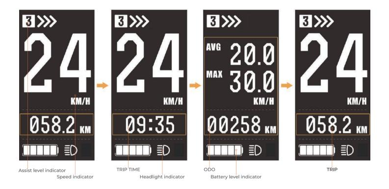
In the power-on state, short press the setting button to switch between TRIP/TRIP TIME/AVG/MAX/ODO
