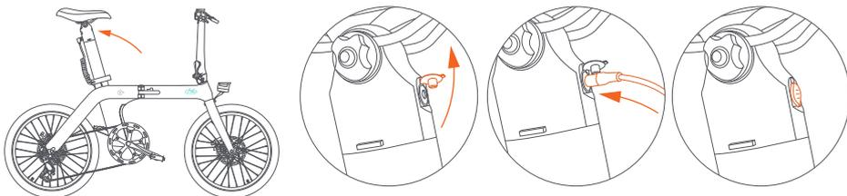
1. Charging connection: Connect the charging interface of the charger to the charging port, then connect the power plug of the charger to the power socket.
