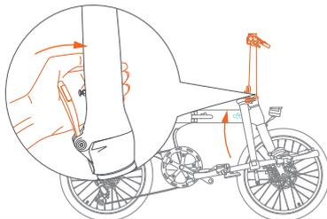
① Open the quick release, adjust the handlebar direction upward to loose the wire.
