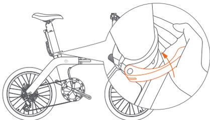
③ Buckle the seat clamp to ensure that the seatpost battery won't slide down
