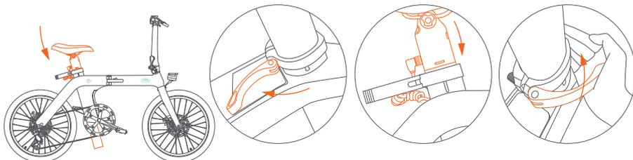
Lift the seat clamp upward, to keep it in open status. Gently press down the seatpost to the bottom. Press down the seat clamp to keep it in closed status.
