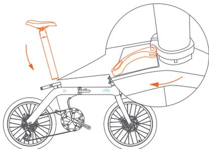
① Open the seat clamp, insert the seatpost battery.
