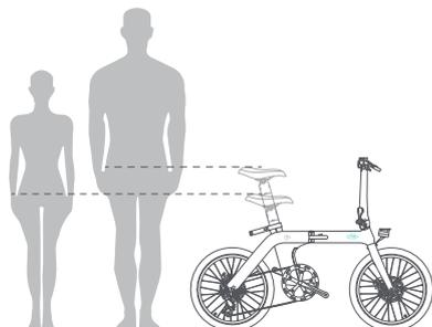
② Adjust the seatpost battery to suitable height, the recommended height is when the saddle is level with the user's pelvis when standing naturally.
