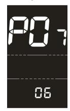
Setting interface of magnetic steel number of speed measuring sensor
