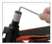
Loosen the screws to remove the front fork sleeve.
