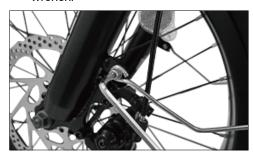
Plug in the headlight. Locate the two sides of the orange, three-pin headlight connector, carefully align the internal pins and notches and external arrows, then press directly together without twisting to fully seat the connection.
