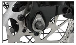
Line up the fork with the axle at the center of the wheel. Make sure there's a spacer between the fork and wheel on each side. Install safety hook, gasket, and nut in turn.
