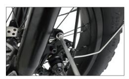
Remove the nut, washer, and bolt at the bottom of the front fork slide the fender through the fork. Reattach the lower fender screws.
