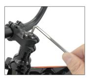
3 Tighten the screws to fix the stem in place.
