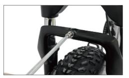
Take out the fender, remove the nut, washer and bolt at the top of the front fork.
