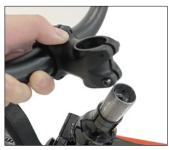
Take out the stem and insert it into the front frame.
