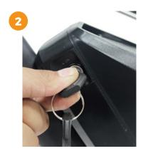
Carefully slide the battery upwards and lift it off the frame. Note: the battery weighs around 5.7 lbs and should be handled with care.
