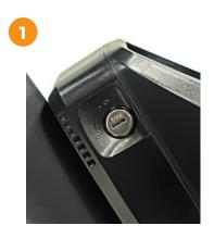
Ensure the battery is off. Align the key port with the appropriate off position by inserting the key into the keyport and rotating to align the key with the off icons.
