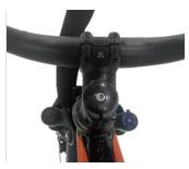
4 After making sure the stem is aligned with the direction of the tire, Tighten the clamping screws below the stem to fix the direction.
