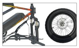
Locate the quick-release lever. Open the lever and remove the thumb nut, safety hook, and cone spring (opposite the lever). Keep the washer, another safety hook, and cone spring in place on the lever side.
