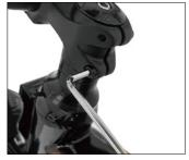
Tighten the screws to fix the handlebar in place.
