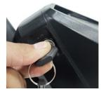
The battery can be removed from the bicycle for charging. To remove the batter, see the previous remove battery section for details, and then carefully pull the battery up until the battery detaches from the receptacle.
