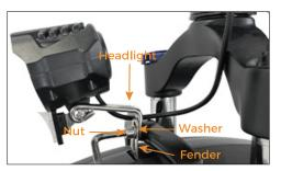
Take out the headlights and screws (including1xBolt,1xWasher, and 1xNut) Slide the fender through the fork. Reattach the bolt, washers.fender, headlight, and nut (in that order) with 8mm wrench.
