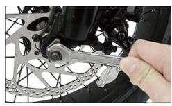
3 Tighten the nut onto the fork with No.15 wrench.
