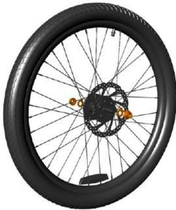
2.3.6 Clamp the front wheel with the front fork and lock the front wheel screw with a 15mm open-end wrench.
