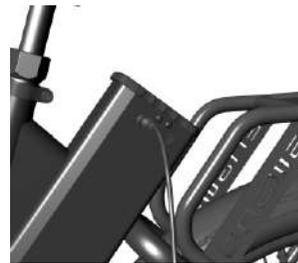
5.3.2 When inserting the AC end of the charger into the AC power socket, at this time the charger indicator light is red, charging begins at this time;
