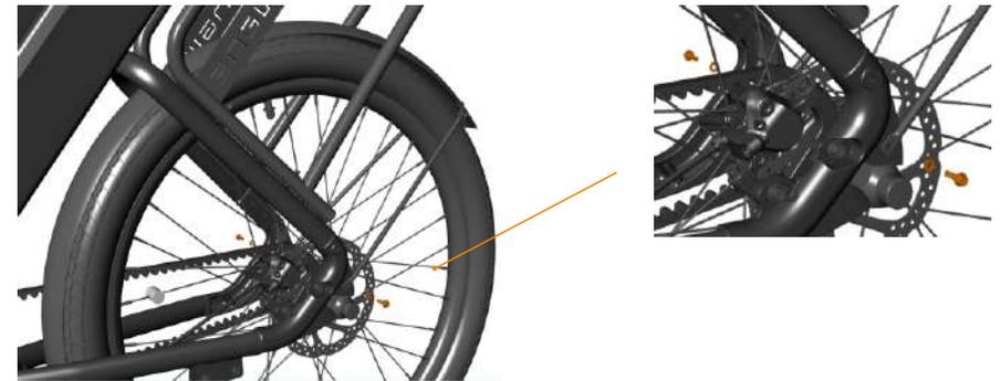
2.3.8 Take the cargo rack out of the cardboard box, remove the wrapped foam, align it with the installation hole as shown in the figure below, and tighten the screw with an 4 hex wrench.
