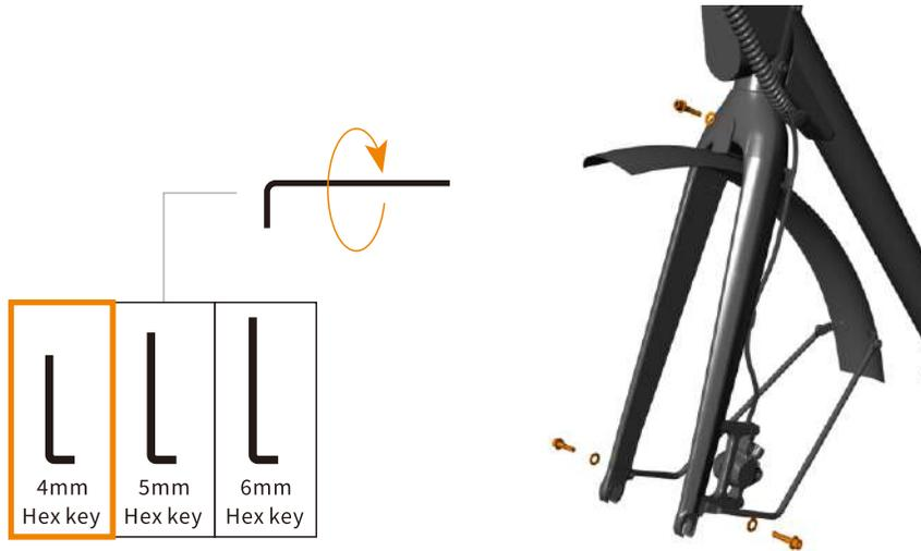
2.3.5 Place the nut and washer on the front wheel as shown in the figure below, following the sequence.
